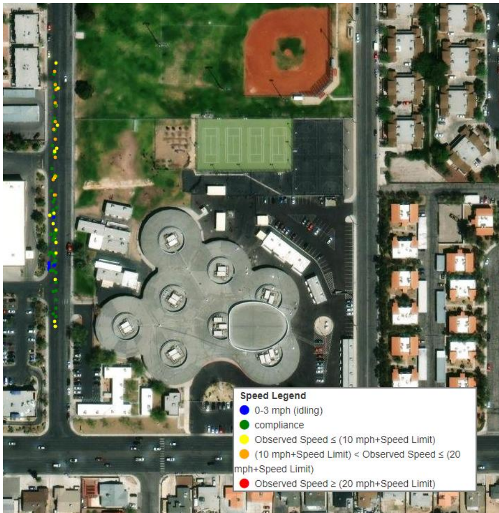
Figure 3.8. Southbound Trajectory Waypoints on Warnock Road during School Zone Speed Control Period
